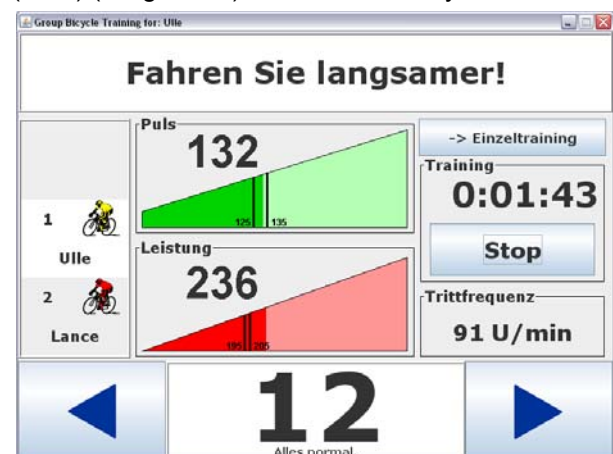
Figure 2. For each cyclist, heart rate ("Puls"), power ("Leistung"), cadence ("Trittfrequenz") and time as well as the position are monitored on the touch screen of the UMPC. On top, feedback as well as advice from the TCTS is displayed (e.g. "Drive slowly"/"Fahren Sie langsamer"). The bottom line shows the current rate of perceived exhaustion on the Borg scale. With the two buttons on the left and the right, cyclists can adjust their rating.
